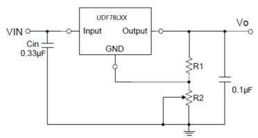
Fig.3 Adjustable Output Regulator
