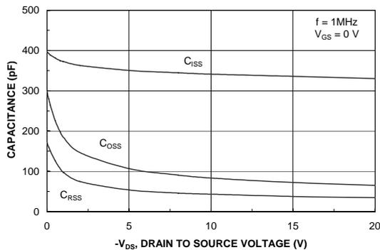
Figure 8. Capacitance Characteristics.
