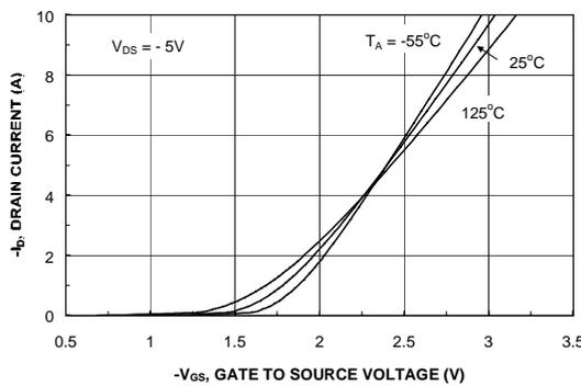
Figure 5. Transfer Characteristics.
