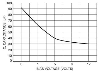
Figure 5. Typical Diode Capacitance (SM12)
