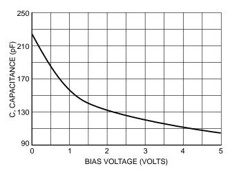
Figure 4. Typical Diode Capacitance (SM05)
