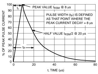
Figure 3. 8/20 µs Pulse Waveform
