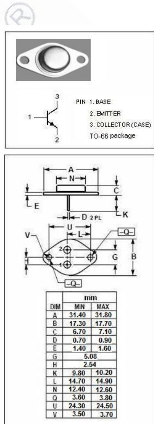
**isc Silicon NPN Power Transistor****2N4912****ELECTRICAL CHARACTERISTICS****T<sub>c</sub>=25°C unless otherwise specified**
