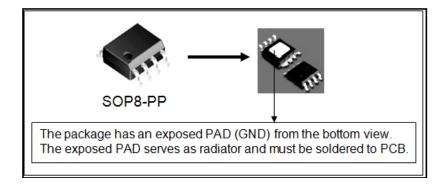
Figure 1. Package Types of TD1484A
