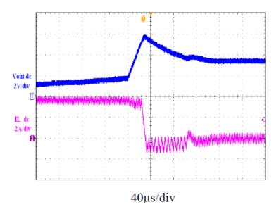
Figure16 Short Circuit Recovery
