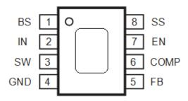
Figure 2 Pin Configuration of TD1484A(Top View)
