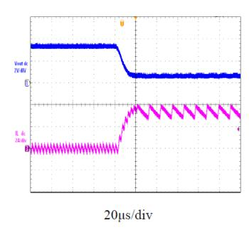
**Figure 15 Short Circuit Protection**
