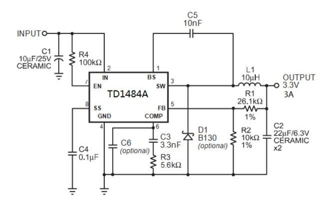
Fig17. TD1484A with 3.3V Output,  $22\mu F/6.3V$  Ceramic Output Capacitor
