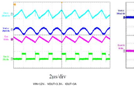
Figure 13. Heavy Load Operation
