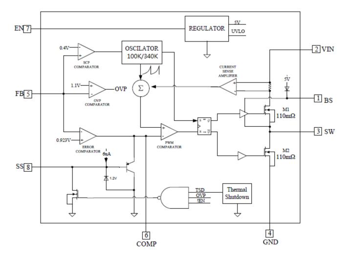
Figure 3 Function Block Diagram of TD1484A
