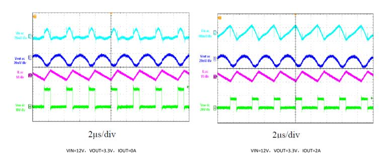
Figure 11 Light Load Operation
