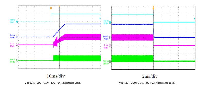
Figure 9. Startup through Enable
