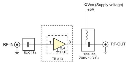
**Fig 1**. Block Diagram of Test Circuit used for characterization. (DUT soldered on Mini-Circuits Test Board TB-313) Gain, Output power at 1dB compression (P1 dB) and output IP3 (OIP3) are measured using R&S Network Analyzer ZVA-24. Noise Figure measured using Agilent's N5242A PNA-X microwave network analyzer.
