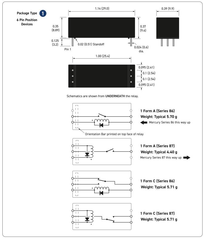
**Important:** Where the optional internal diode is fitted or for all Form B types, the correct coil polarity must be observed as shown by the + symbol on the schematics.
