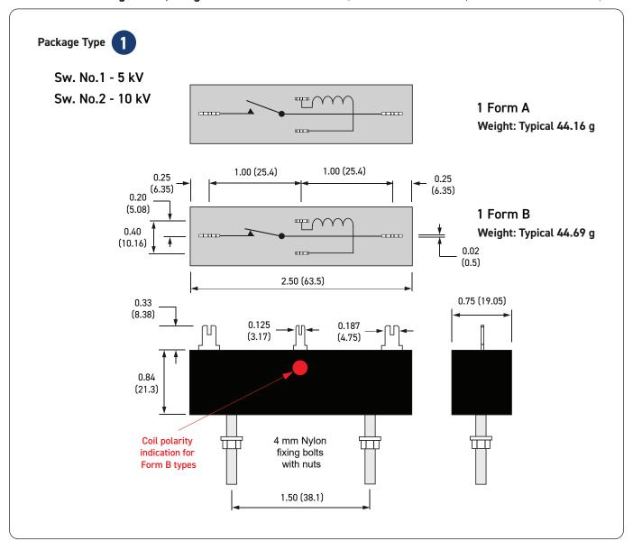
**Important:** For all Form B types, the correct coil polarity must be observed. The positive connection is shown by the red spot on the package.
