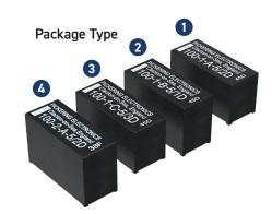
The Pickering Series 100 is a complete range of Single-in- Line (SIL) reed relays primarily intended for direct drive from 4000B CMOS or NMOS logic or similar low current sources. The mercury wetted relays in the range may be driven directly from TTL logic.
