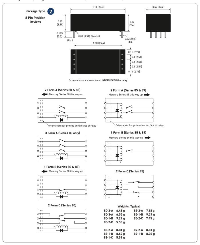
**Important:** Where the optional internal diode is fitted or for all Form B types, the correct coil polarity must be observed as shown by the + symbol on the schematics.
