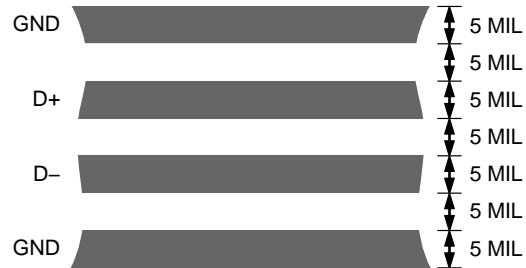
Figure 34. Typical Arrangement of Signal Tracks
