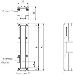
01) When removing the end cap, there is the lamp output terminal (top) or the power supply terminal (bottom).
