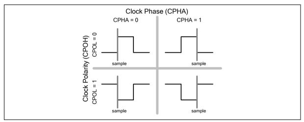
Figure 6.9-4 SPI Clock Formats
