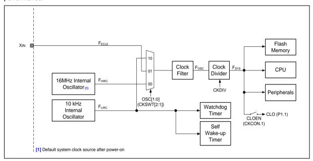
Figure 6.2-1 Clock System Block Diagram
