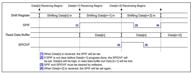
Figure 6.9-7 SPI Overrun Waveform
