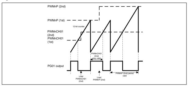
Figure 6.11-3 PWM Edge-aligned Type Waveform
