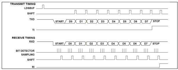
Figure 6.8-2 Serial Port Mode 1 Timing Diagram
