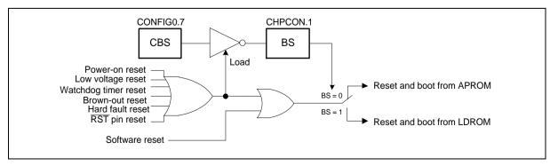
Figure 6.2-3 Boot Selecting Diagram
