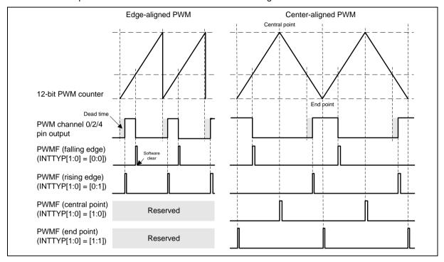
Figure 6.11-7 PWM Interrupt Type
