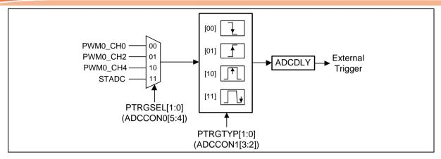
Figure 6.12-2 External Triggering ADC Circuit
