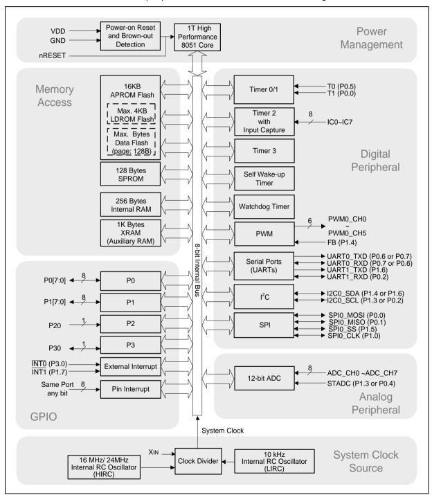
Figure 5.1-1 Functional Block Diagram
