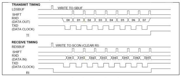
Figure 6.8-1 Serial Port Mode 0 Timing Diagram
