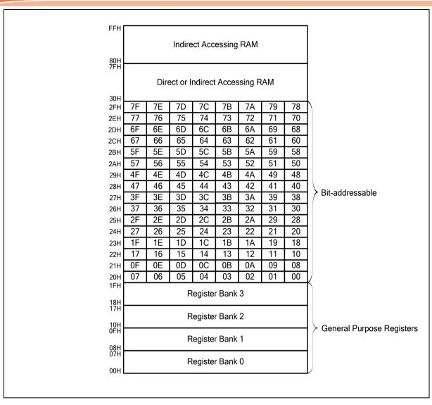
Figure 6.1-6 Internal 256 Bytes RAM Addressing
