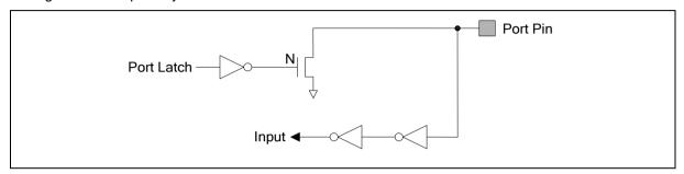
Figure 6.4-4 Open-Drain Mode Structure
