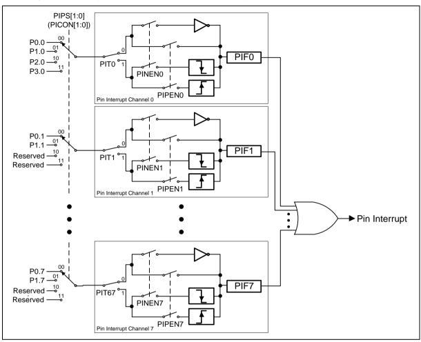
Figure 6.4-5 Pin Interface Block Diagram
