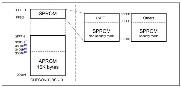
Figure 6.1-2 SPROM Memory Mapping And SPROM Security Mode
