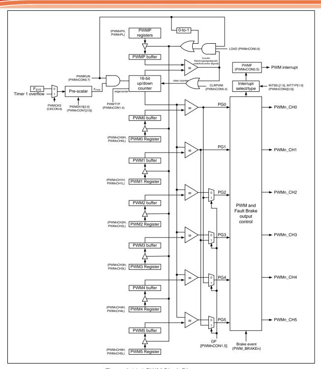
Figure 6.11-1 PWM Block Diagram
