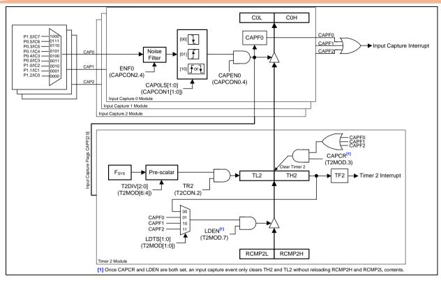
Figure 6.5-6 Timer 2 Auto-Reload Mode Block Diagram
