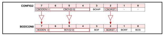
Figure 6.1-4 CONFIG2 Power-On Reset Reloading
