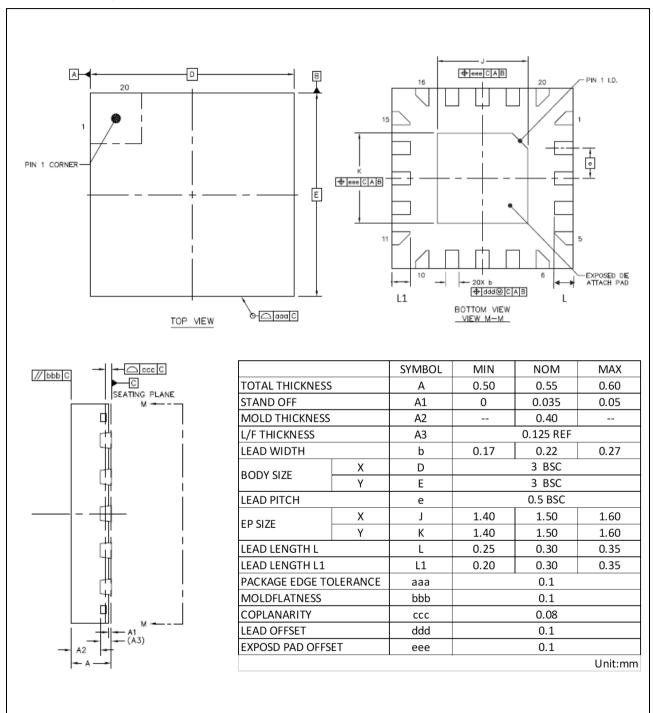
Figure 9.2-1 QFN-20 Package Dimension for MS51XB9AE
