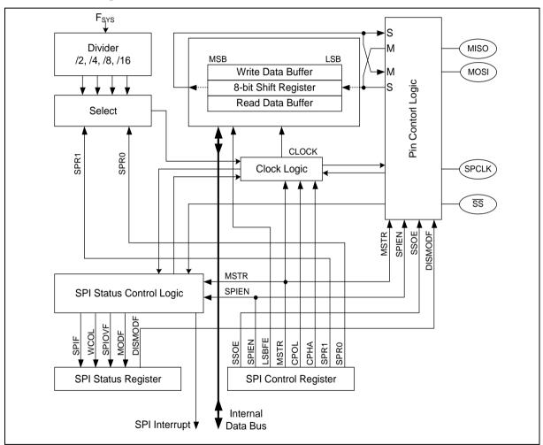
Figure 6.9-1 SPI Block Diagram
