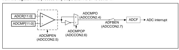
Figure 6.12-3 ADC Result Comparator
