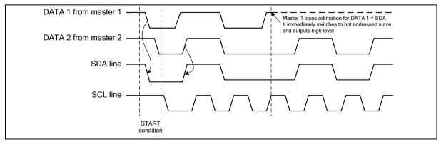
Figure 6.10-8 Arbitration Procedure of Two Masters
