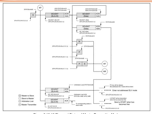
Figure 6.10-10 Flow and Status of Master Transmitter Mode
