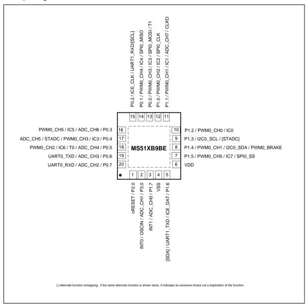
Figure 4.1-2 Pin Assignment of QFN-20 Package
