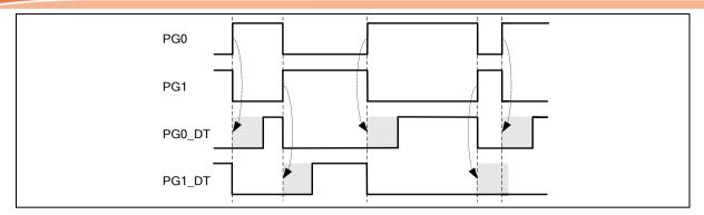
Figure 6.11-5 PWM Complementary Mode with Dead-time Insertion
