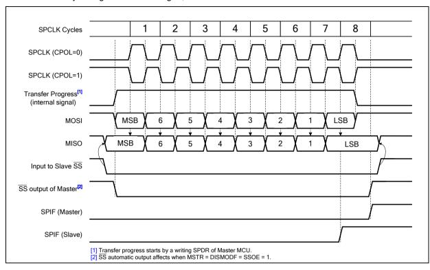
Figure 6.9-5 SPI Clock and Data Format with CPHA = 0
