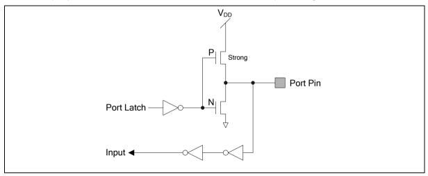
Figure 6.4-2 Push-Pull Mode Structure
