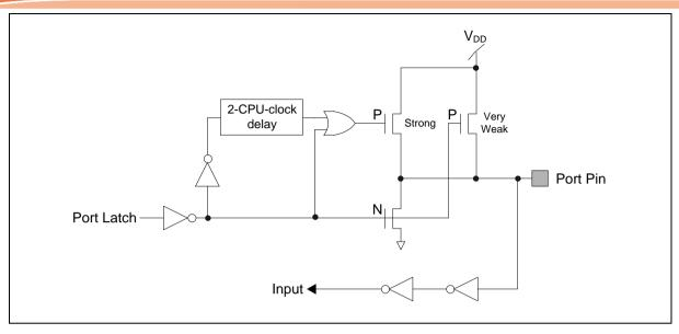
Figure 6.4-1 Quasi-Bidirectional Mode Structure
