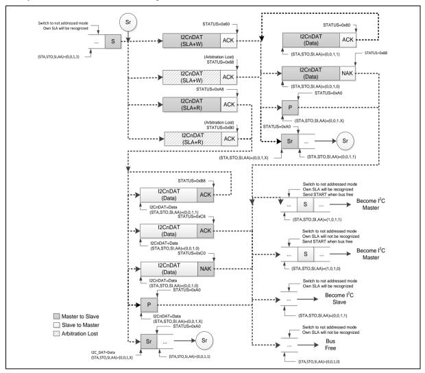
Figure 6.10-12 Flow and Status of Slave Receiver Mode
