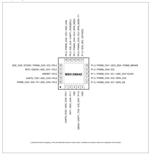
Figure 4.1-1 Pin Assignment of QFN-20 Package
