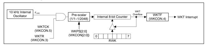
Figure 6.7-1 Self Wake-Up Timer Block Diagram
