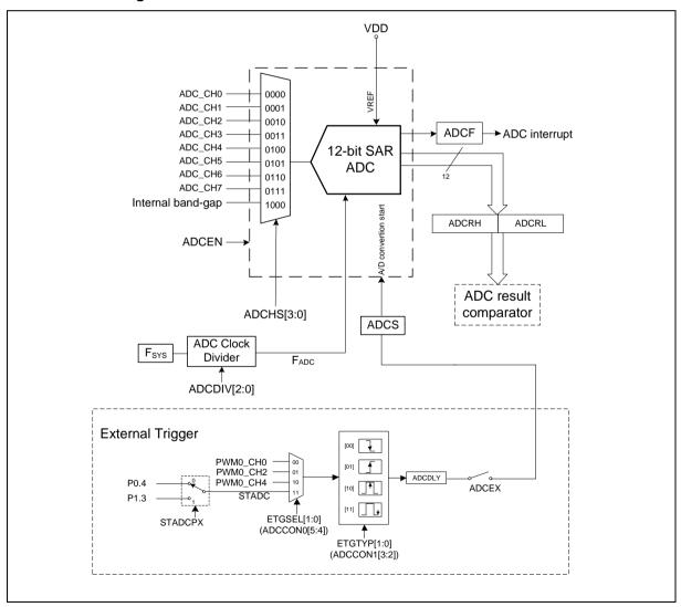
Figure 6.12-112-bit ADC Block Diagram
