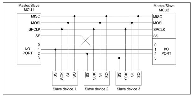
Figure 6.9-2 SPI Multi-Master, Multi-Slave Interconnection
