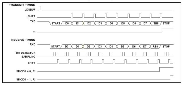
Figure 6.8-3 Serial Port Mode 2 and 3 Timing Diagram
