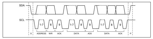
Figure 6.10-6 Data Format of One I<sup>2</sup>C Transfer
