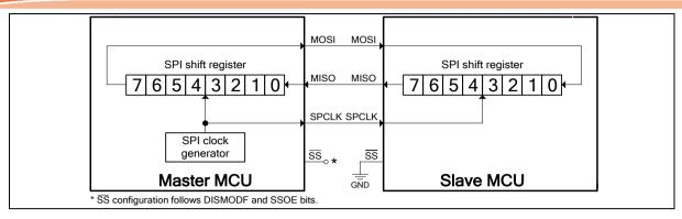
Figure 6.9-3 SPI Single-Master, Single-Slave Interconnection
