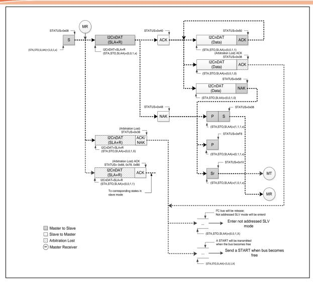
Figure 6.10-11 Flow and Status of Master Receiver Mode
