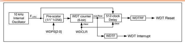
Figure 6.6-1 WDT as A Time-Out Reset Timer
