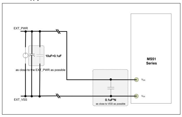
Figure 7.1-1 NuMicro® MS51 Power supply circuit
