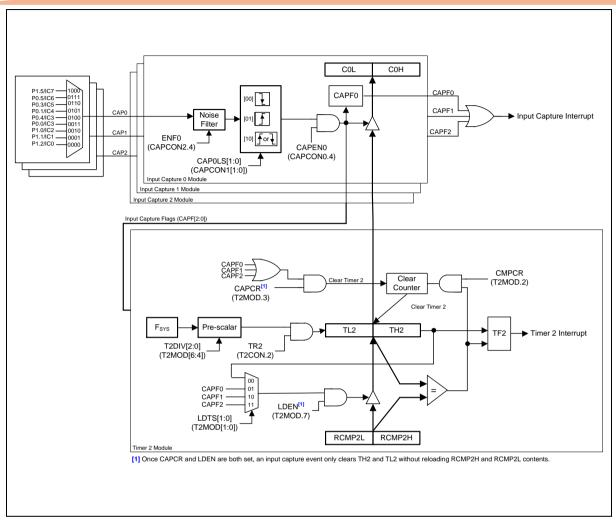
Figure 6.5-5 Timer 2 Full Function Block Diagram
