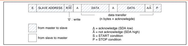
Figure 6.10-4 Master Transmits Data to Slave by 7-bit
