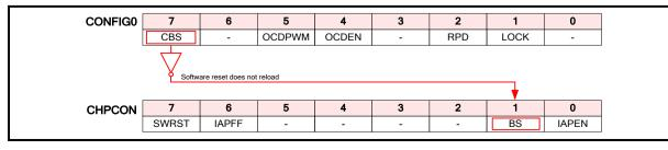
Figure 6.1-3 CONFIG0 Any Reset Reloading
