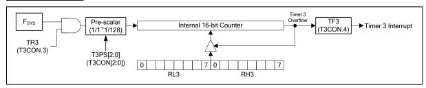
Figure 6.5-8 Timer 3 Block Diagram
