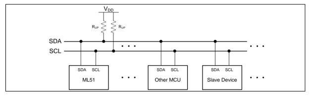
Figure 6.10-1 I<sup>2</sup>C Bus Interconnection
