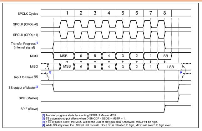
Figure 6.9-6 SPI Clock and Data Format with CPHA = 1
