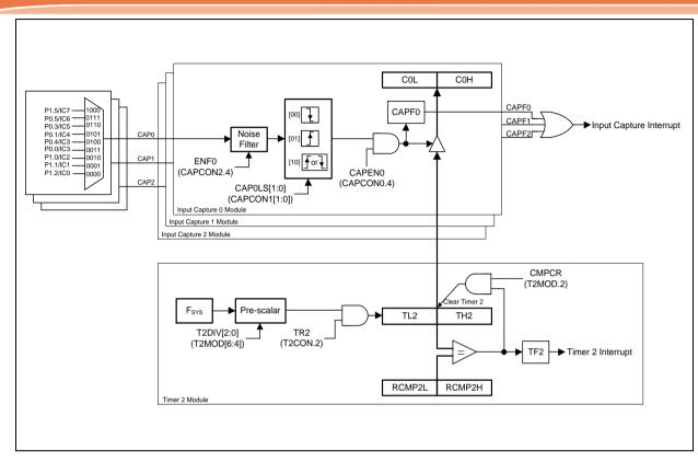
Figure 6.5-7 Timer 2 Compare Mode Block Diagram
