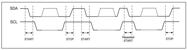
Figure 6.10-3 START, Repeated START, and STOP Conditions
