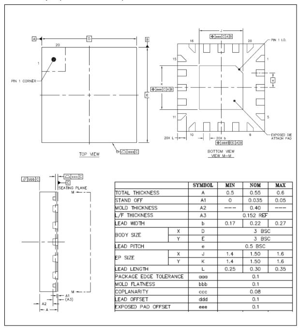
Figure 9.3-1 QFN-20 Package Dimension for MS51XB9BE
