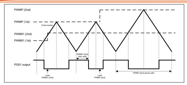
Figure 6.11-4 PWM Center-aligned Type Waveform
