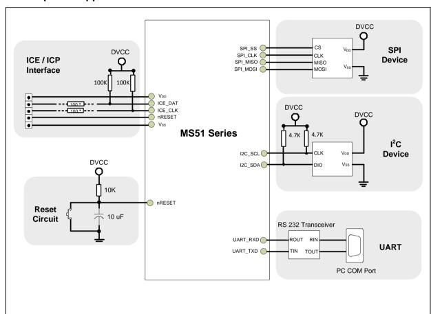
Note 1: It is recommended to use 100 k $\Omega$  pull-up resistor on both ICE\_DAT and ICE\_CLK pin.
