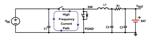
Figure 19. High Frequency Current Path
