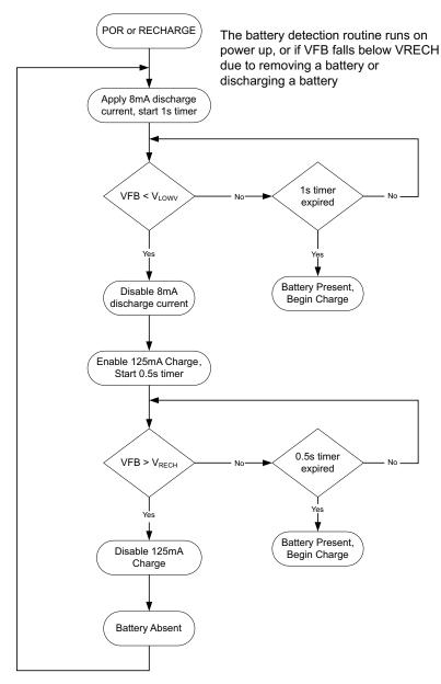
Figure 8. Battery Detection Flowchart
