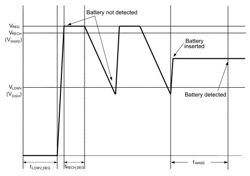
Figure 9. Battery-Detect Timing Diagram
