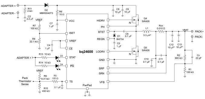
$V_{IN} = 28 \text{ V}$ , BAT = 5-cell Li-Ion,  $I_{charge} = 3 \text{ A}$ ,  $I_{pre-charge} = I_{term} = 0.3 \text{ A}$
