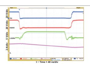
Figure 14. Continuous-Conduction-Mode Switching Waveforms
