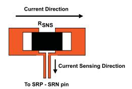
Figure 18. Sensing Resistor PCB Layout
