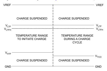
Figure 6. TS Pin, Thermistor Sense Thresholds
