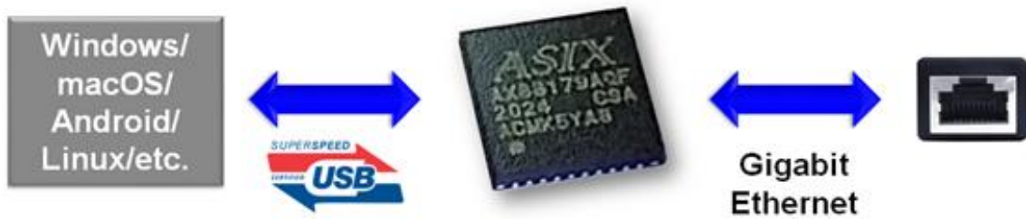
Figure 0-1: AX88179A Typical Applications Diagram
