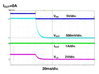
Figure 16. Power Off through EN Waveform
