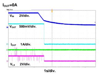
Figure 12. Power Off through VIN Waveform
