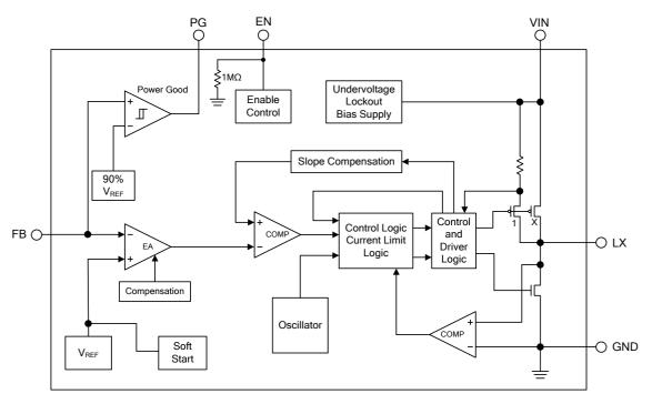
Figure 3. Block Diagram of PL5903
