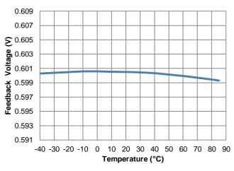
Figure 7. Feedback Voltage vs. Temperature
