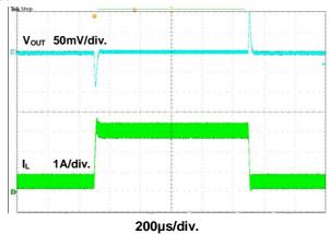
Figure 18. Load Transient Waveform
