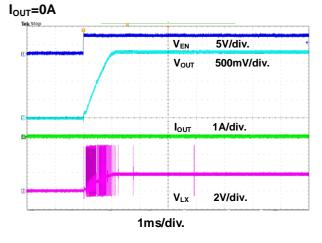
Figure 14. Power On through EN Waveform
