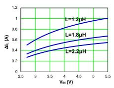
$V_{OUT}$ =1.8V,  $F_{OSC}$ =1MHz
