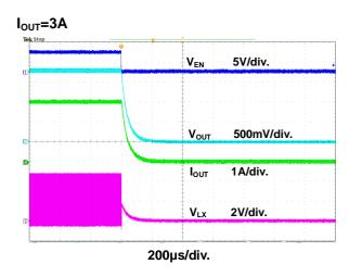
Figure 17. Power Off through EN Waveform
