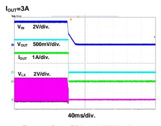
Figure 13. Power Off through VIN Waveform
