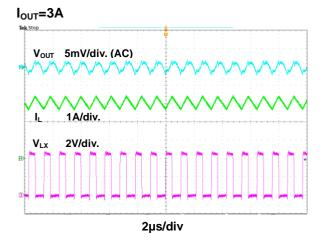
Figure 9. Steady State Waveform
