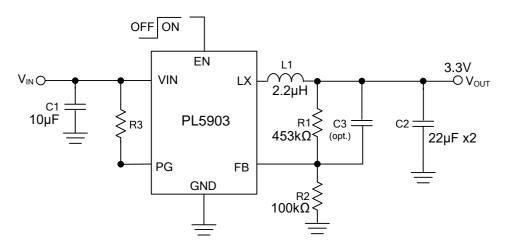
Figure 2. Schematic Diagram
