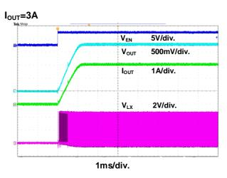
Figure 15. Power On through EN Waveform
