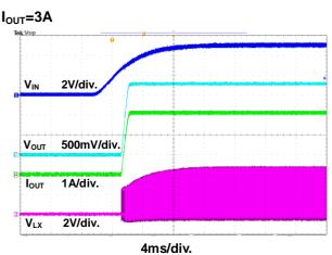
Figure 11. Power On through VIN Waveform
