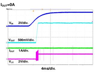
Figure 10. Power On through VIN Waveform
