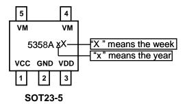
Figure 1. PIN Configuration
