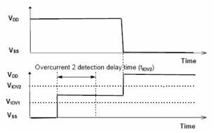
Figure 4. Overcurrent delay time
