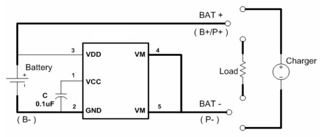
Fig 6 PL5358 in a Typical Battery Protection Circuit
