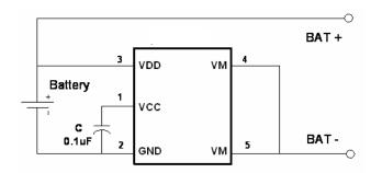
Figure 2. Typical Application Circuit
