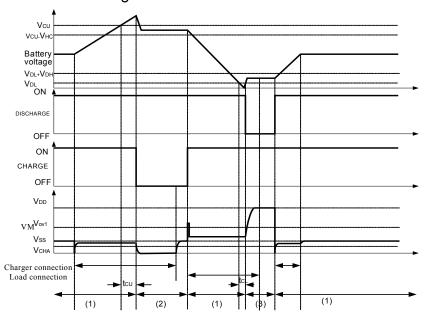
Figure 5-1 Overcharge and Overdischarge Voltage Detection
