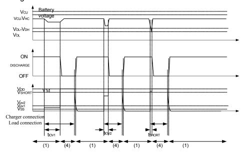
**Figure5-2 Overdischarge Current Detection**
