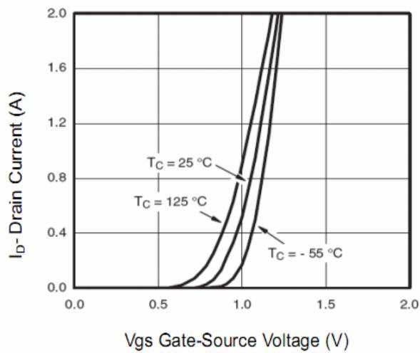
Figure 7 Transfer Characteristics
