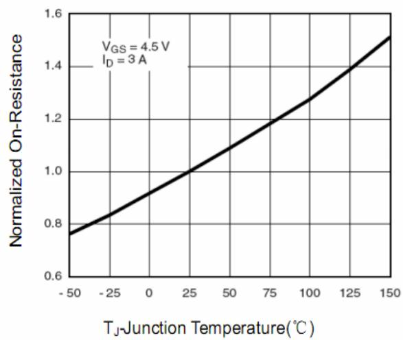
Figure 8 Drain-Source On-Resistance
