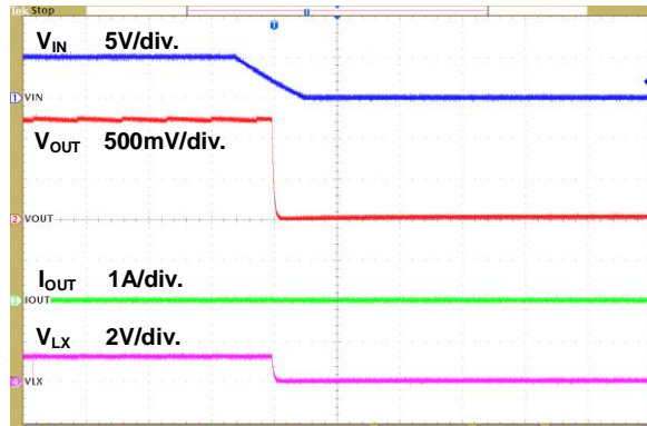
Figure 10. Power Off through VIN Waveform
