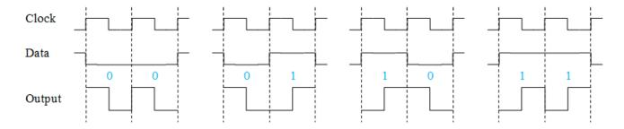
All commands sent to the OPB9010 are sent via the CAL/STAT pin. Each command must first begin with the syncing nibble (1100). The first two bits "11" allow the decoder to detect the data clock. The second two bits are a check for detection of the "00" data. The third two bits determine the command being sent. The available commands are:
