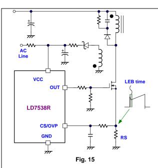
A leading-edge blanking (LEB) time is included in the input of CS pin to prevent the false-trigger from the current spike.
