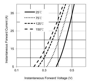
Fig.3 - Typical Forward Voltage Characteristics
