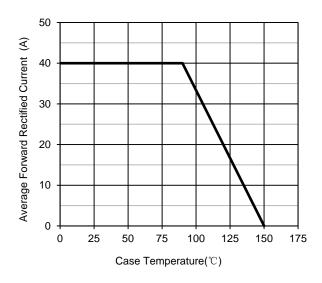
Fig.1 – Forward Current Derating Curve
