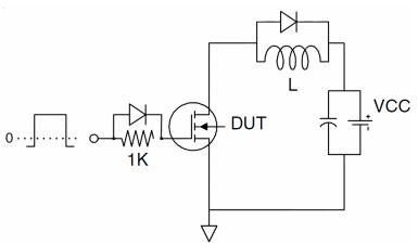
3) Switch Time Test Circuit:
