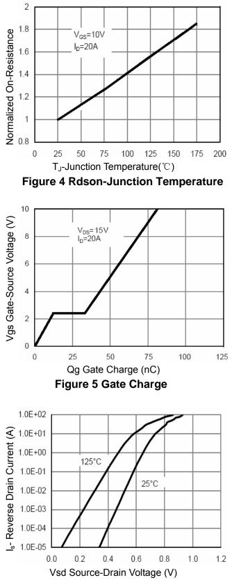
Figure 6 Source- Drain Diode Forward
