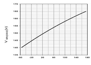
$T_{J}- Junction \ Temperature({}^{\circ}\!C)$  Figure 12 BV<sub>DSS</sub> vs Junction Temperature
