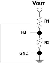
For adjustable voltage mode, the output voltage is set by an external resistive voltage divider according to the following equation:
