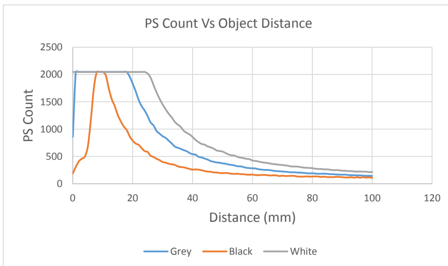
Figure 4.2: PS performance across distance VDD 3V, 9mA, 32pulses, with others in default settings.
