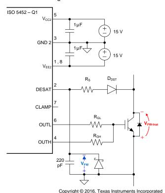
Figure 55. DESAT Pin Protection with Series Resistor and Schottky Diode
