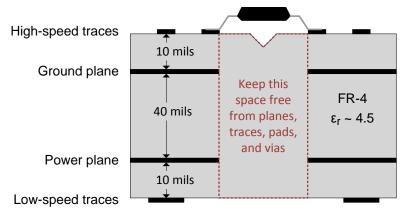
Figure 60. Recommended Layer Stack
