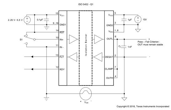
Figure 47. Common-Mode Transient Immunity Test Circuit
