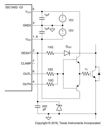
Figure 57. Current Buffer for Increased Drive Current
