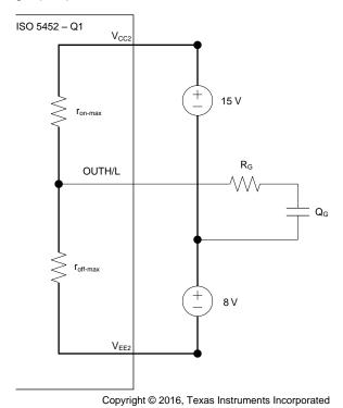
Figure 56. Simplified Output Model for Calculating Pol-WC
