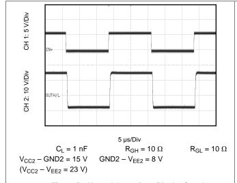
Figure 58. Normal Operation - Bipolar Supply
