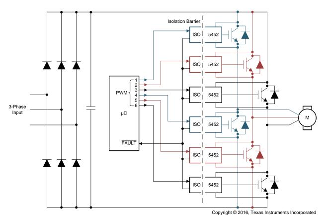
Figure 48. Typical Motor Drive Application
