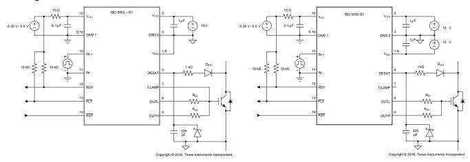
Figure 49. Unipolar Output Supply
