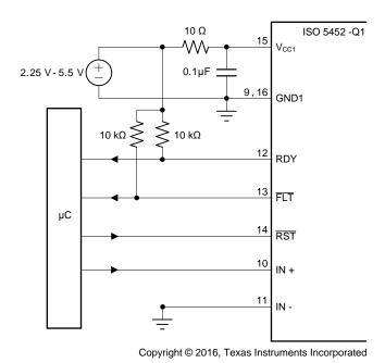
Figure 51. FLT and RDY Pin Circuitry for High CMTI
