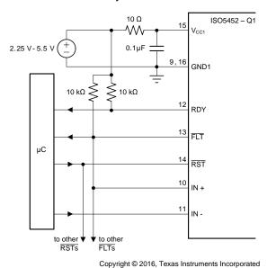
Figure 53. Global Shutdown With Inverting Input Configuration
