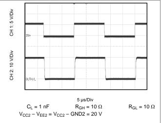
Figure 59. Normal Operation - Unipolar Supply
