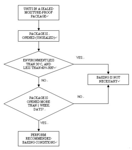
If the parts are not stored in dry conditions, they must be baked before reflow to prevent damage to the parts. Baking should only be done once
