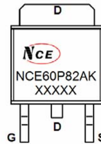
Marking and pin assignment
