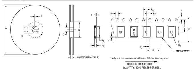
В С D G N Α Min. Max. Min. Max. Min. Max. Min. Max. Ref. Ref. 2.5 (.098) 330 1.5 12.8 13.5 20.2 102 326 16.5 (13.002)(.059)(.795)(.650) $\overline{(4.016)}$ (12.835)(.504)(.531)
