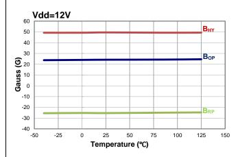
**Switch Points Bop and Brp vs Temperature**
