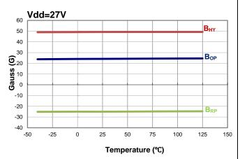
Switch Points Bop and Brp vs Temperature
