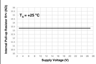
Internal Output Pull-up Resistor vs Supply Voltage
