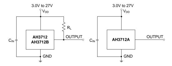
Note: 4. C<sub>IN</sub> is for power stabilization and to strengthen the noise immunity, the recommended capacitance is 10nF ~ 100nF. R<sub>L</sub> is the pull-up resistor.
