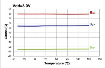
**Switch Points Bop and Brp vs Temperature**
