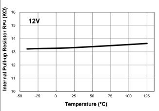
Internal Output Pull-up Resistor vs Temperature
