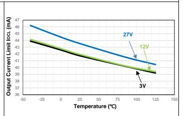
**Output Current Limit vs Temperature**
