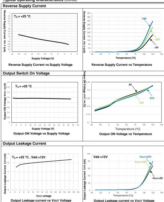
Output Leakage current vs Vout Voltage
