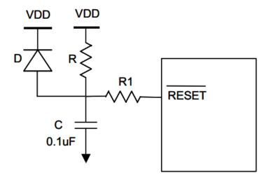
Figure 20 Block Diagram of Reset Application
