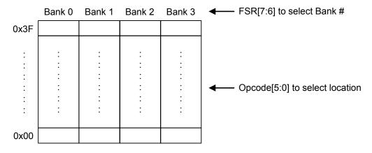
Figure 4 Direct Addressing Mode of Data Memory Access
