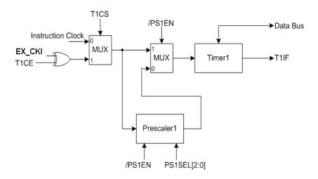
Figure 11 Block Diagram of Timer1
