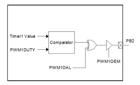
Figure 13 PWM1 Block Diagram
