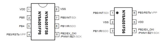
Figure 1 Package pin assignment
