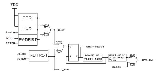
Figure 19 Block diagram of on-chip reset circuit
