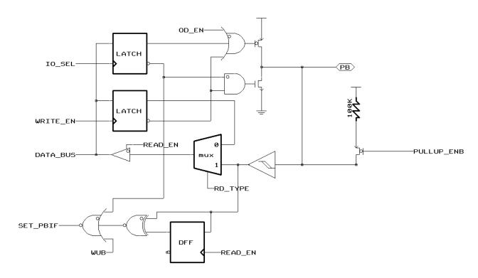
Figure 9 Block Diagram of PB4/PB5
