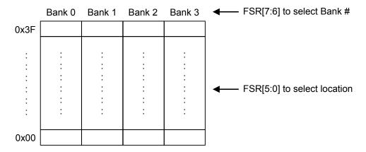
Figure 3 Indirect Addressing Mode of Data Memory Access
