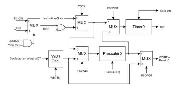
Figure 10 Block Diagram of Timer0 and WDT
