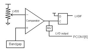
Figure 16 LVD block diagram
