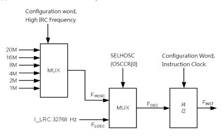
Figure 17 Oscillation Configuration of NY8A051F
