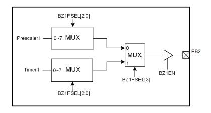
Figure 14 Buzzer1 Block Diagram
