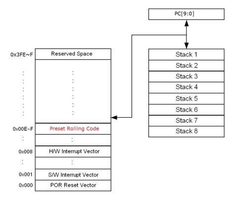
Figure 2 Program Memory Address Mapping
