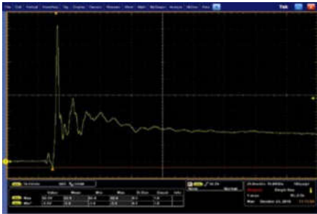
Positive 8kV contact per IEC 61000-4-2
