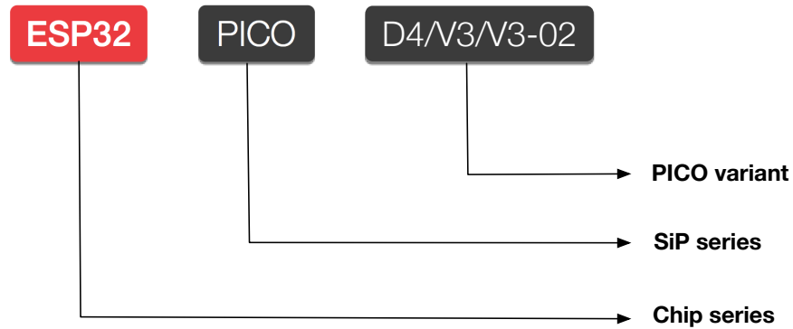
Figure 2: ESP32-PICO Series Nomenclature
