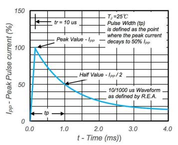
Fig.3 - Pulse Waveform
