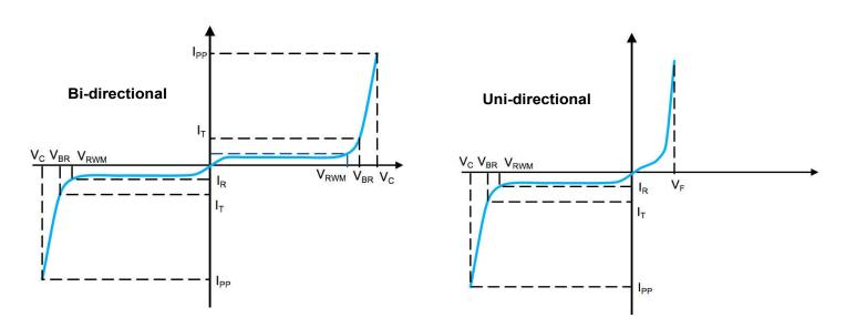
P<sub>PPM</sub> Peak Pulse Power Dissipation - Max power dissipation
