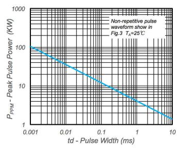
Fig.1 - Peak Pulse Power Rating
