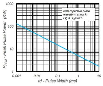
Fig.1 - Peak Pulse Power Rating
