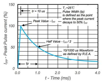
Fig.3 - Pulse Waveform
