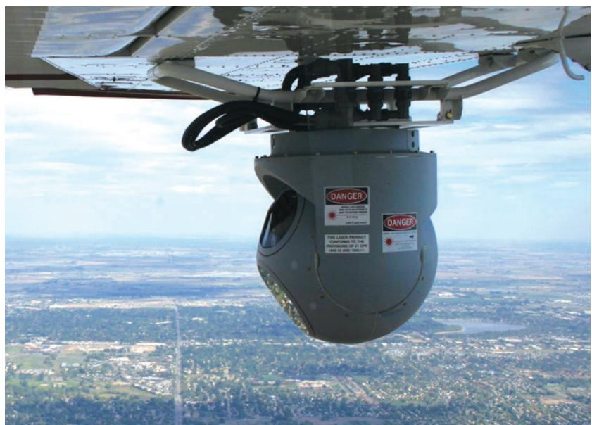
Cameras mounted on aircraft require special stabilization to create clear images or motion pictures, surveillance, and other applications. The KVH DSP-3000 is an essential part of many of these systems.
