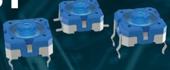
The RACON ST fits into your operating system as if it were tailor-made. The product family offers the right tactile switch for every project: The RACON 8 ST and RACON 12 ST series differ in their dimensions and operating forces. SMT as well as THT versions are available for both.
