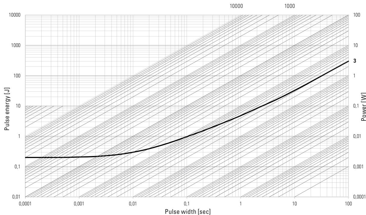
This curve is only valid for the resistance value R005. The shape of the curve in the range below 0.1 sec will be different for other resistance values. Therefore a separate qualification should be made for pulse power close to the above curve.
