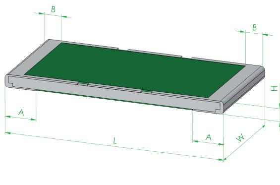
Layout if TC < 20 ppm/K is required for R in between 30 and 80 mOhm
